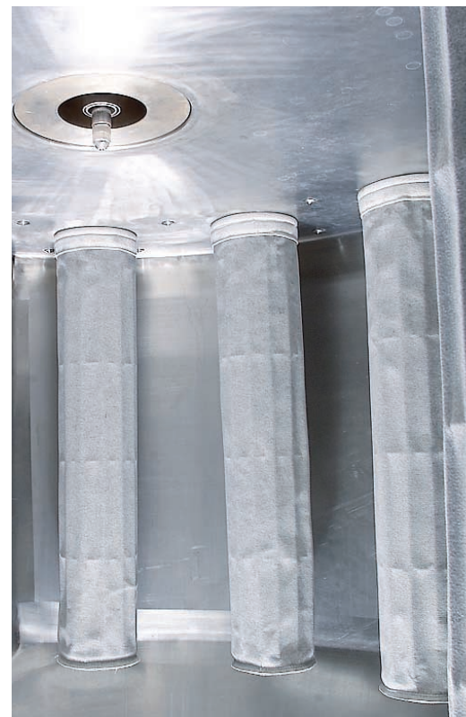
Integrated filters reduce space requirements. Whether using the SANICIP™ cleaning system or not, an integrated filter will enhance performance for a long range of products.
