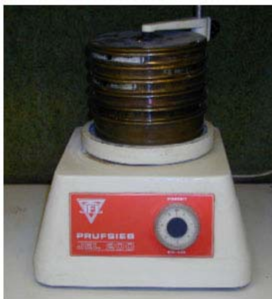
Fig. 1 Shaker for sieves.
