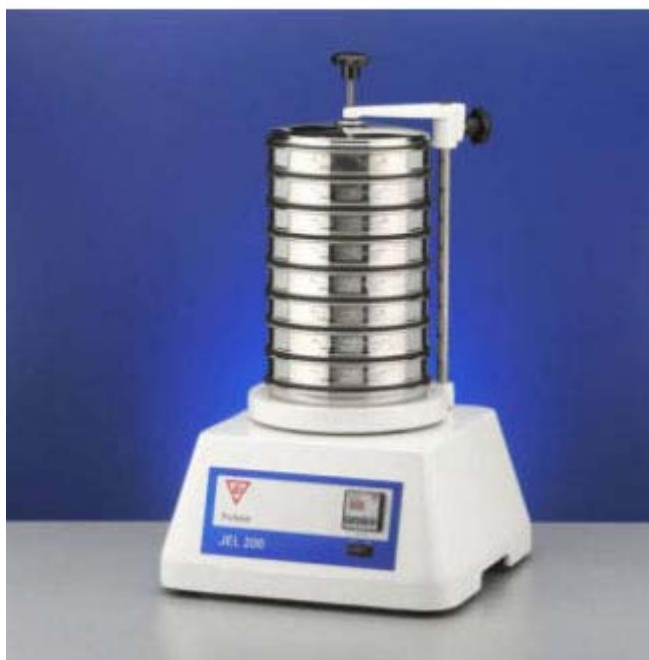
Fig. 1 Shaker for sieves.
