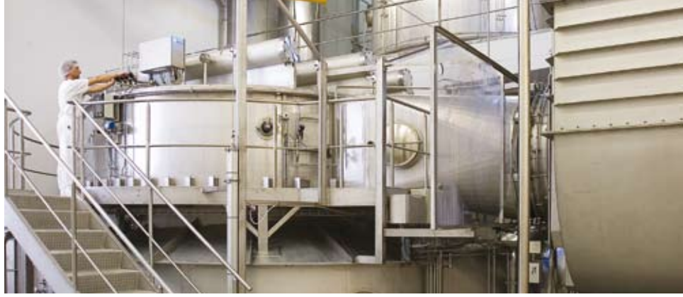
The top of a SANICIP™ bag filter
