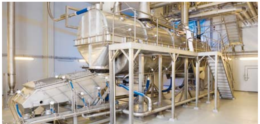
VIBRO-FLUIDIZER™ and sieve with side-mounted CIP nozzles
