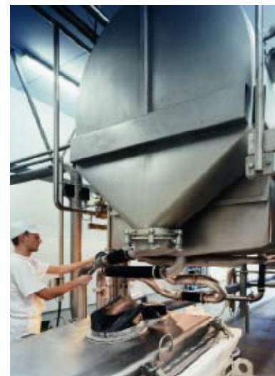
Preparing the VIBRO-FLUIDIZER™ for CIP cleaning by placing a tunnel which returns the cleaning liquid to the CIP kitchen
