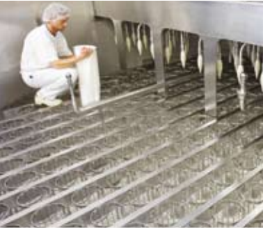
The patented SANICIP™ bag filter with top cover open
