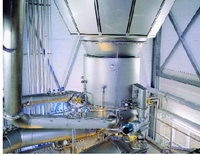
Chamber cone, integrated fluid bed and sieve with CIP nozzles
