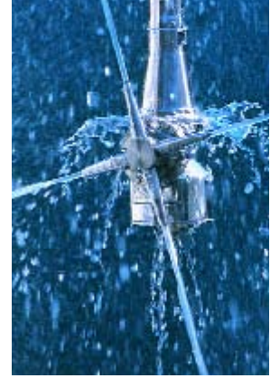
Jet liquid nozzle for cleaning of the drying chamber surface
