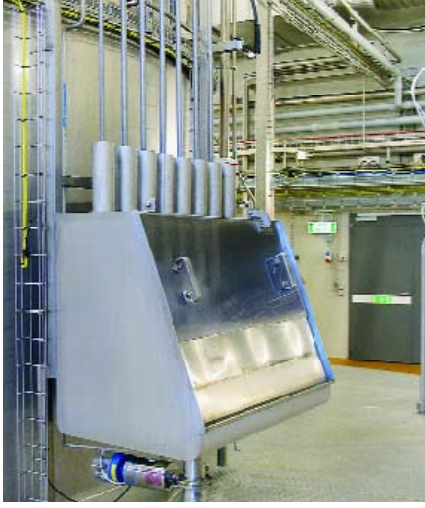
High pressure atomizer nozzles ready for CIP cleaning. All nozzles lances and nozzle heads are placed in a special stand for cleaning
