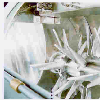
Inlet duct and rotating intensifier
