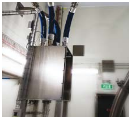
Powder diverter valve enabling remote control of the powder flow
