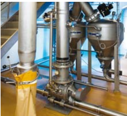
Powder transport by HEPA filtered air to avoid contamination of the powder
