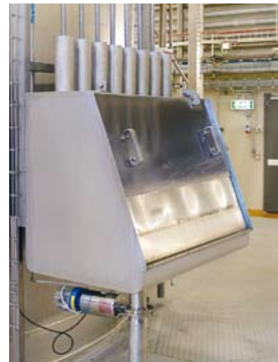
Cleaning of nozzle lances and/or rotary atomizer is performed in a specially designed CIP stand, which is included in the CIP circuit for the feed line. Disassembly of nozzle lances and the high-pressure feed line/flexible high-pressure hose is therefore unnecessary
