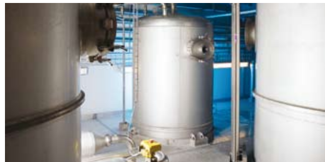
Flash regenerative vessels with no heat transfer surface reduces steam consumption. When the same principle is used instead of traditional tubular pre-heaters, 20 hours continuous production is possible with low mesophile and thermophile growth
