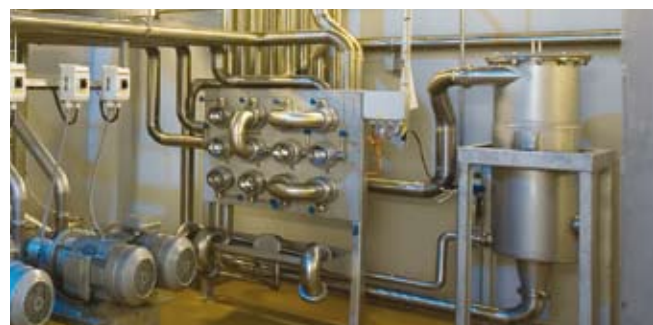
Hydro-cyclone. A self-cleaning in-line filter removes sludge during CIP and gives full protection against blockage of the distribution system
