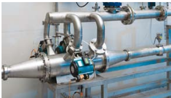
Tangential swirl heater for controllable direct steam injection to final heating temperature makes 20 hours continuous operation possible
