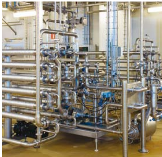
Concentrate heat treatment in a tubular heat exchanger with no moving parts and a corrugated heat transfer surface. The heating is achieved using hot water in a counter-current flow. This results in a low \Delta t and minimum 20 hours of operation even at high temperatures
