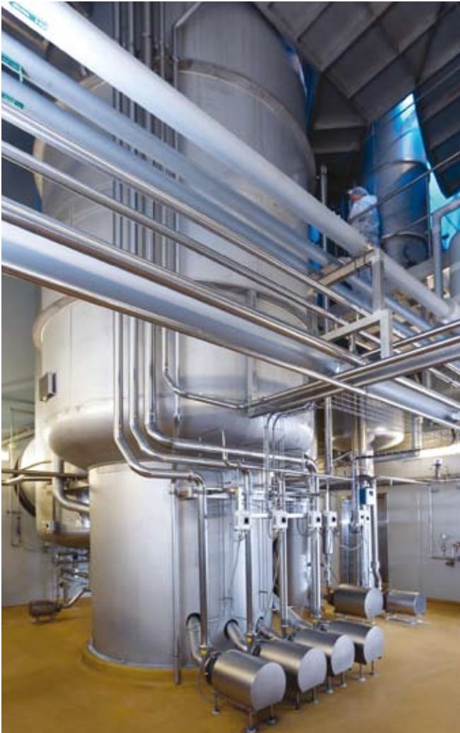
Wrap-around separator with rounded corners improves efficiency. The products' contact to the evaporator's surface is reduced and CIP is done easily
