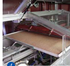
Freeze drying: Tray going into the CONRAD™ freeze dryer
