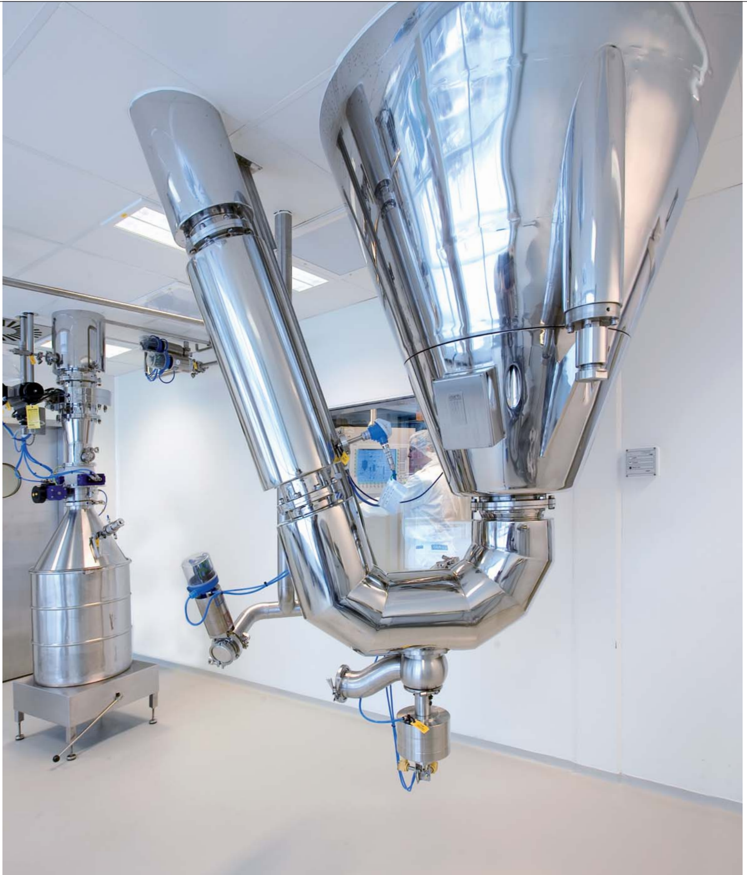
From GEA Niro Pharma Test Station in Copenhagen: GMP suite with a PSD-4 spray dryer in closed-cycle mode
