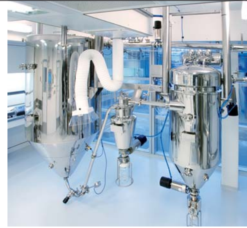
PSD-1 drying chamber, cyclone and bag filter. Nominal drying gas rate: 80 kg/h
