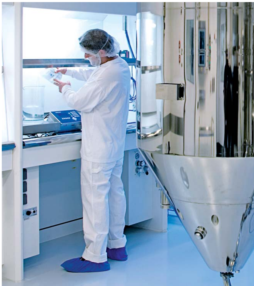
From GEA Niro Pharma Test Station in Copenhagen: GMP suite with a PSD-1 spray dryer in closed-cycle mode
