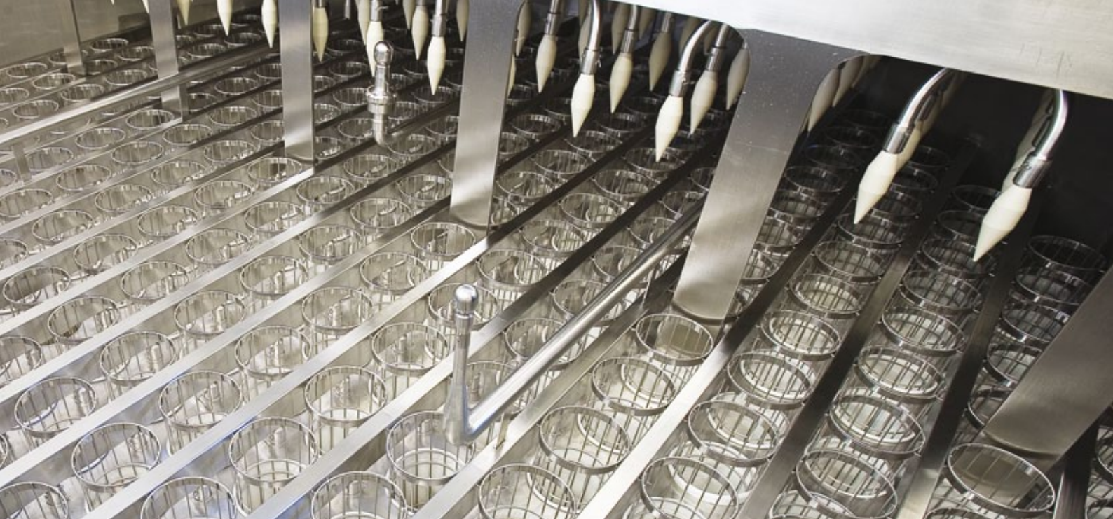
Multiple cyclones can be replaced by just one SANICIP™ bag filter
