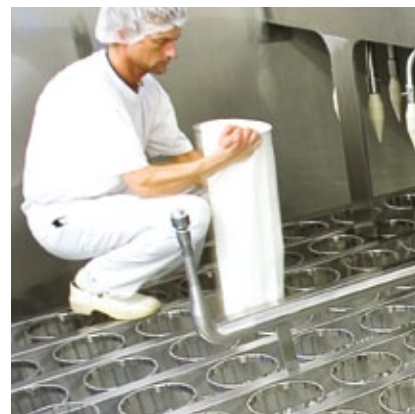
The cages are easily removed, bags are easily changed, and cages are quickly put back in place
