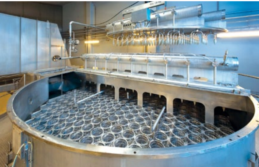
The top of SANICIP™ bag filter is designed for easy access to the bags. The larger bag filter sizes are supplied with a two-section top. This design reduces the required building height and the load on the hoist beam
