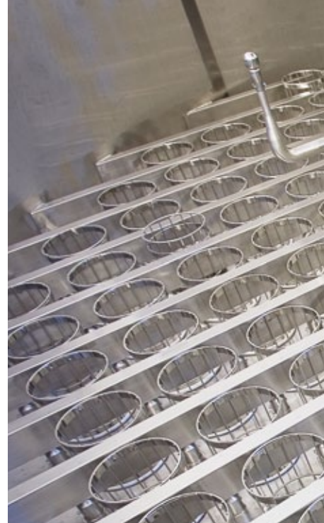
The jet nozzles, all valves and connections are placed in the top cover, meaning free access for maintenance
