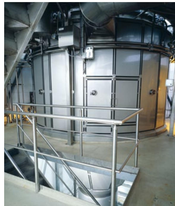
The IFD™ dryer with the filter bags integrated in the drying chamber
