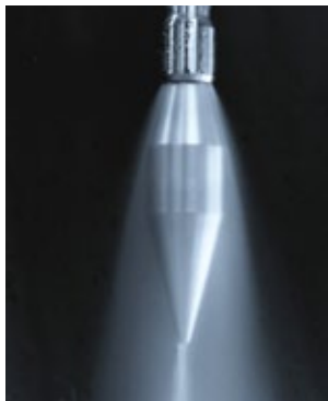
During CIP liquids are sprayed from the jet nozzles
