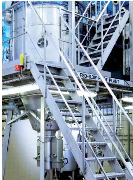
FSD™-6.3 with triple chamber static fluid bed. Installed in GEA Niro Test Center, Copenhagen. Drying chamber size: Ø 1600x800 mm, 40° cone.
