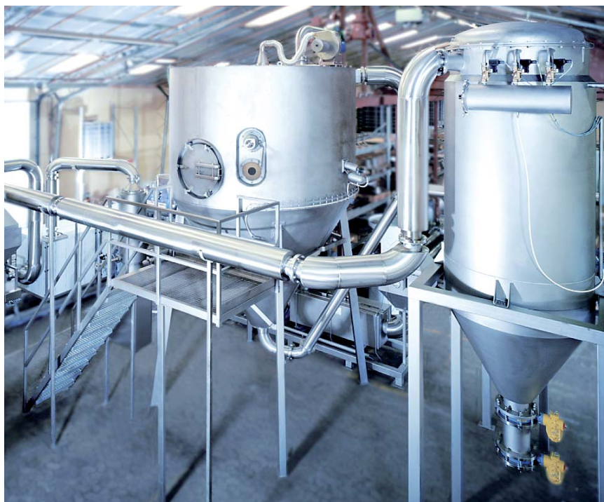
VSD-12.5-CC spray dryer with a rotary atomizer and bag filter. Closed-cycle design using nitrogen as drying gas. Drying chamber size: Ø 2500x1500 mm, 60° cone.
