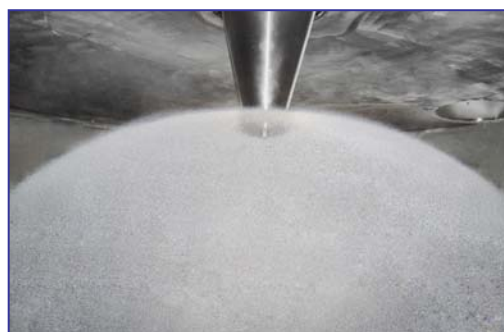
Rotary atomization at chamber top
